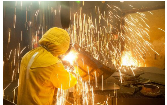
CENTRACO Cyclife – Thermal cutting prior to melting
